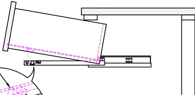
Once the back hook is connected gently lower the drawer onto the front metal pin.
