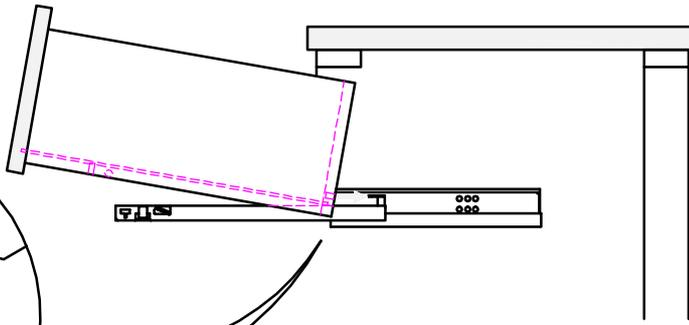
Extend the runner all the way out. Put the drawer onto them then hold both the runners with your hands, lift the drawer up with your thumbs and push to hook the drawer at the end of the runner.
